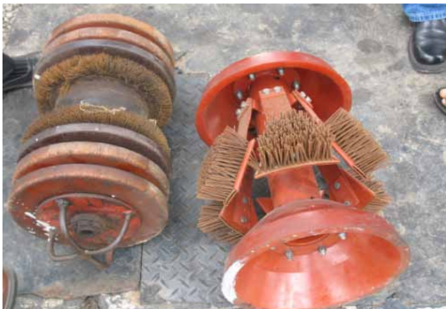
Sample of a pig which is inserted into a pipeline
